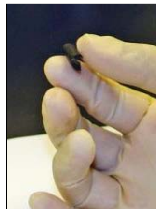
A paper battery can be bent, and springs back into shape.
