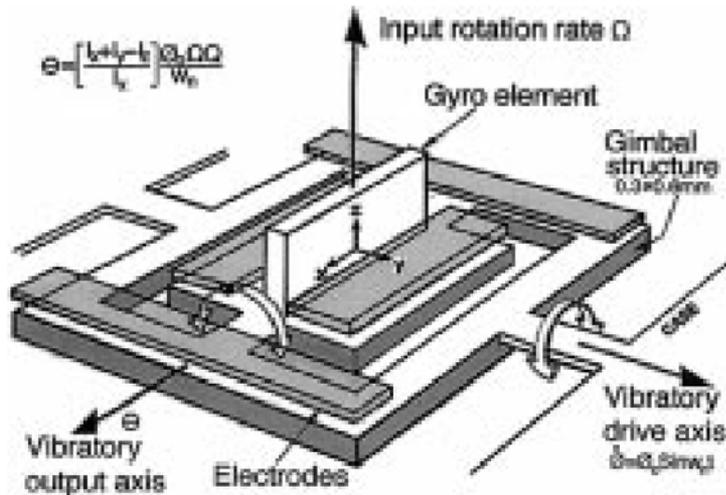
**Fig. 10.** Draper's first silicon micromachined double-gimbal vibratory gyroscope (1991) [100].
