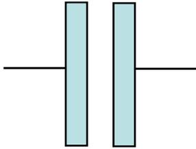
Consider charging up these plates through a large resistor  $R$ , so that the characteristic time  $RC$  is much longer than the timescale of the motion you want to detect.
