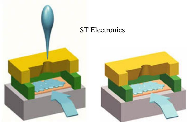
True 2400 dpi printing = 10 micron droplets ~ few micron nozzles.
