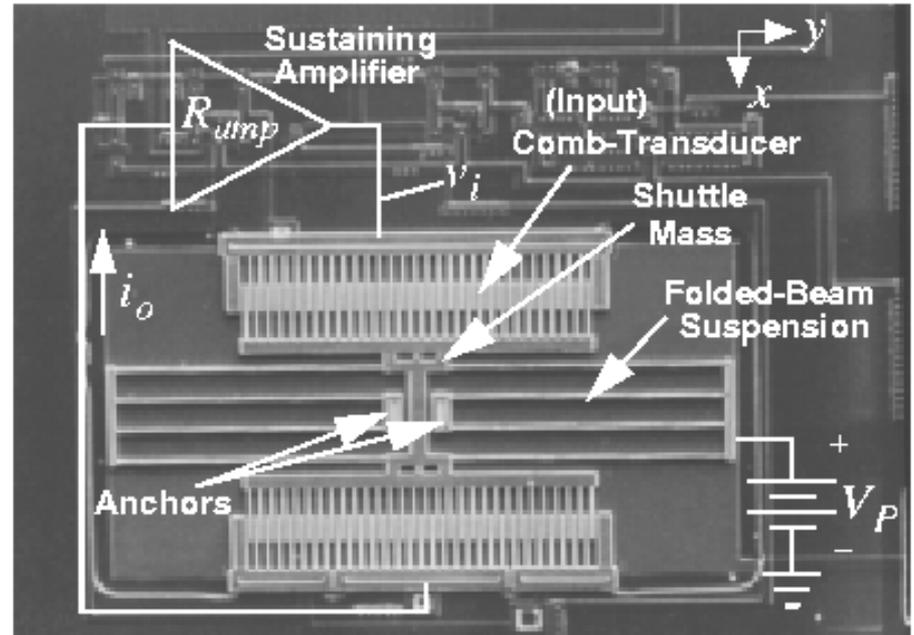
To run the device as an oscillator, this signal is amplified and applied back to the drive electrode.
