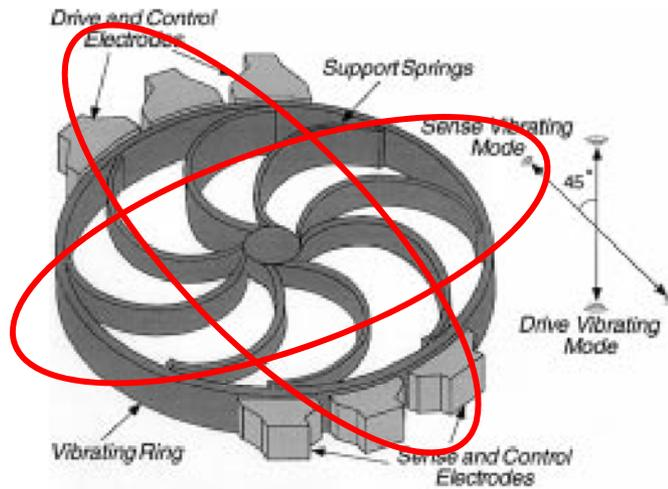
Fig. 15. Structure of a vibrating ring gyroscope.
