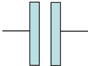
At given voltage,  $F \propto C(V_{dc} + V_0 \exp(-i\omega t))^2$
