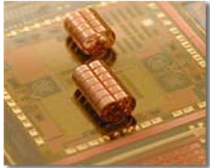
Similarly, use prestressed metal structures to lift components off wafer surface for more movement clearance.
