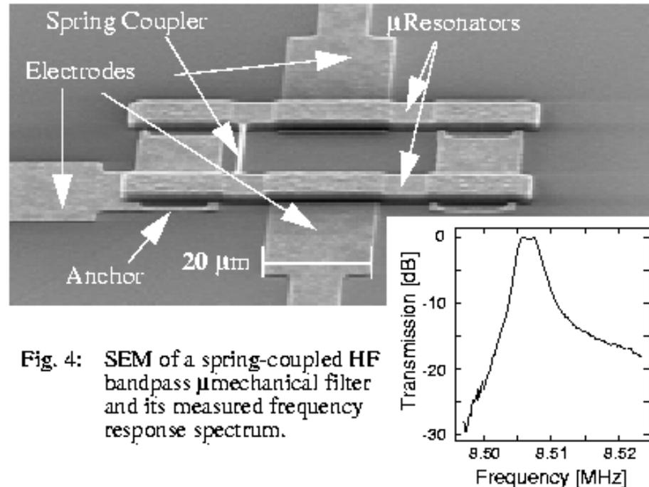
Fig. 4: SEM of a spring-coupled HF bandpass  $\mu$ mechanical filter and its measured frequency response spectrum.
