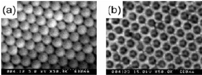
Figure 1. SEM images of polystyrene opal film (a) and SiO<sub>2</sub> inverse opal film (b) prepared from polystyrene spheres with a diameter of 260 nm.
