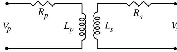
Fig. 1 Circuit diagram of a simplified transformer, including resistance of the wire in the coils.
