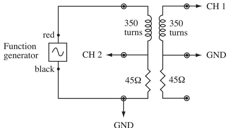
Fig. 3 Wiring diagram for the model transformer, with plug connectors as indicated. The 45 Ω resistors are provided for current measurement. The effective coil resistance is not shown.
