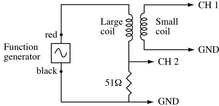
Fig. 2. Circuit for measuring induced voltage. The large coil has 552 turns and an average radius of 0.12 m. The smaller pickup coil has 200 turns and an average radius of 0.033 m.
