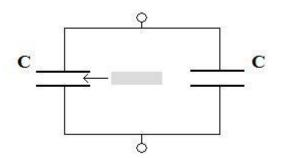
A dielectric of dielectric strength  $\kappa$  is now inserted to entirely fill the gap between the plates of one capacitor. The energy shared by the pair of capacitors is –
