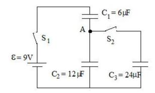
III. (25 pts) Consider the circuit shown below, where switches  $S_1$  and  $S_2$  are open and  $C_1$ ,  $C_2$  and  $C_3$  are uncharged.
