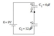
(b) What is now the potential at point A? (Take the potential on the negative terminal of the source of emf to be 0V).
