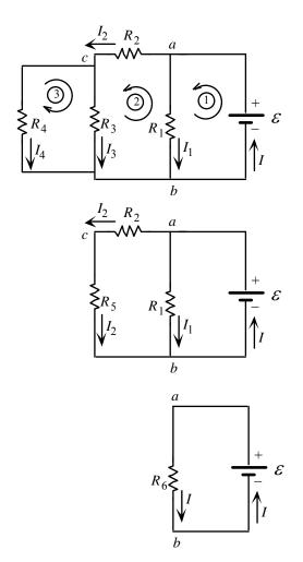
$$V_{cb} = I_2 R_5 = (0.113 \text{ A})(33.3 \Omega) = 3.75 \text{ V}.$$
