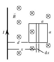
$$\Phi_B = \iint \vec{B} \cdot d\vec{A} = \iint B \, dA = \int_d^{a+d} \frac{\mu_0 I}{2\pi x} a \, dx$$
