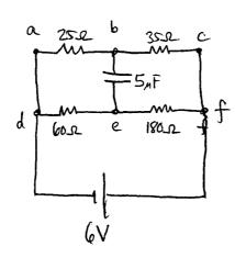
After a very long time the capacitar is fully charged so no current 'flows' thru capacitar.
