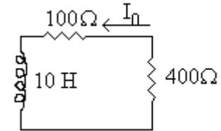
$$V_1 = (100\Omega)(0.25A) = 25V.$$
