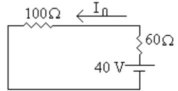
$$I_0 = \frac{V}{R_{eq}} = \frac{40V}{100\Omega + 60\Omega} = 0.25A$$
