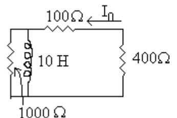
0.25A flowing through the original resistors, but also the power being dissipated through the  $1000\Omega$  resistor, also initially held at 125V, which equals  $\frac{V^2}{R} = \frac{125^2}{1000} = 15.625W$ .
