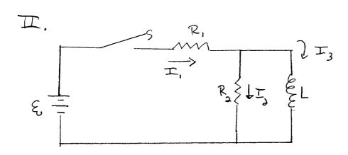
(a) Amnedeately after Sis closed, there is no current through L, since the current in an inductor carrot charge abruptly. R. &R, are in series
