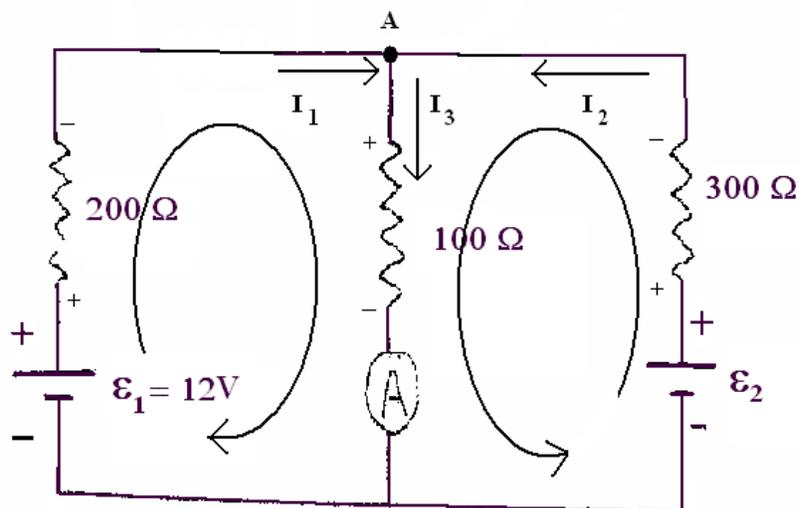
The value of  $\epsilon_2$  can then be determined by applying Kirchoff's Junction and Loop rules. First, the direction of currents are selected and the potential drops across the currents are labeled, consistent with the flow of current (current will flow from the positive, or high end of a resistor to the negative, or low end). Then 3 independent equations can be generated and the results from part (a) applied ( $I_3 = I$  from part (a)).
