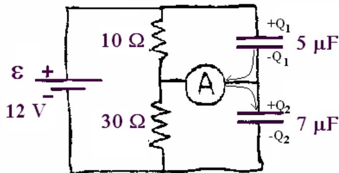
Using this approach, one finds that  $I = V/(R_1 + R_2) = 12V/(10\Omega + 30\Omega) = 0.3A$ . The voltage,  $V_1$ , across the top resistor and capacitor is then  $V_1 = (0.3A)(10\Omega) = 3V$  and the voltage,  $V_2$ , across the bottom resistor and capacitor is  $V_2 = (0.3A)(30\Omega) = 9V$ .
