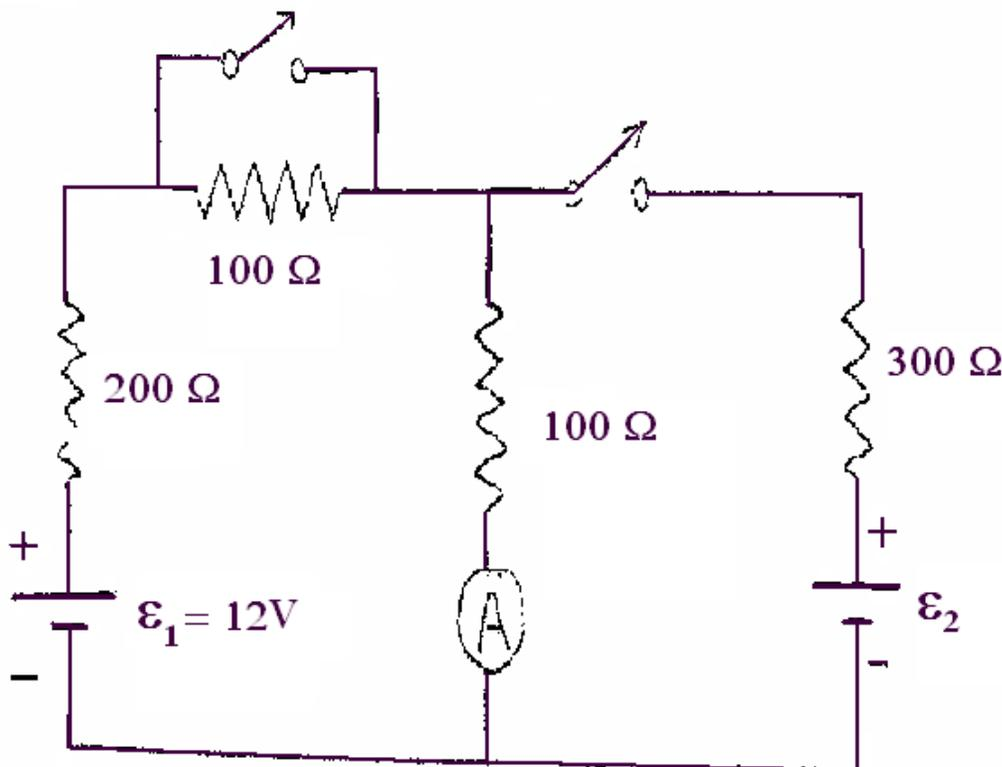
2. (A) In the circuit shown to the right, the current through the ammeter A doubles when switch S is closed. Determine the emf  $\epsilon_2$ .
