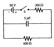
(a) Immediately after the switch is closed, the capacitor acts like a short circuit, that is, a wire with zero resistance. Then the  $600\Omega$  resistor is effectively out of the circuit, and the current is determined only by
