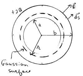
(c) Now suppose a charge +Q is placed in the center of the hollow spherical shell. Draw a spherical Gaussian surface inside the conductor. The field must be zero everywhere inside the conductor, so the net charge enclosed must be zero. Therefore, there must be a charge of -Q in the inner surface of the conductor, at r=a. Since the conductor still has a total charge +2Q, the outer surface r=b must now have a charge of +3Q.
