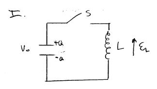
(b) At the charge on the capacitor is a, the Noltago drop across C is  $\stackrel{?}{=}$ . When the switch is closed, I is in the clockwise direction as is  $\frac{dI}{dI}$ . But  $I = -\frac{dQ}{dI}$ , since the charge on C is decreasing. Then Kinchoff's loop equation is
