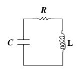
• The overall behavior of the charge oscillation will be affected because the resistance of the wire will cause energy loss (due to heating). The larger the resistance, the faster energy gets dissipated (and the longer the period of oscillation becomes).
