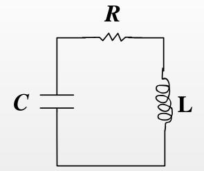
The overall behavior of the charge oscillation will be affected because the resistance of the wire will cause energy loss (due to heating).
