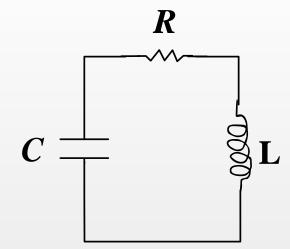
• The overall behavior of the charge oscillation will be affected because the resistance of the wire will cause energy loss (due to heating). The larger the resistance, the faster energy gets dissipated (and the longer the period of oscillation becomes).
