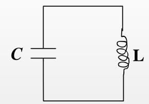
• Start with a *fully charged capacitor* and place it in series with an inductor as shown above.
