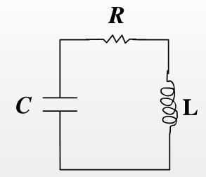
ullet The charge on the capacitor, Q, will undergo simple harmonic motion when the capacitor is directly connected across an inductor.
