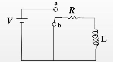
• After a very long time, the switch is thrown into position (b).
