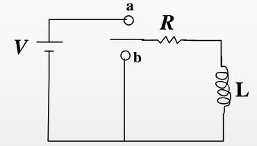
• The magnetic flux through the circuit is initially zero (No current flows in the circuit).
