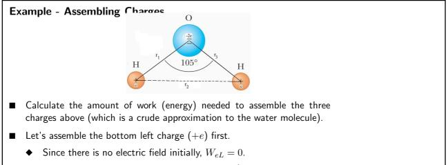
• This charge sets up a electric potential,  $V_1 = \frac{k e}{r}$
