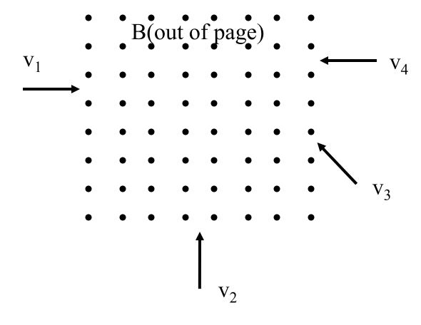
1.  $v_1 = v_2 = v_3 = v_4$ 2.  $v_1 = v_4 > v_3 > v_2$ 3.  $v_1 = v_2 = v_4 > v_3$ 4.  $v_4 > v_3 > v_3 > v_1$ 5. need more info Four particles with the same charge and initial speed are incident on the same region of constant magnetic field, as depicted below. Rank the magnitude of the force due to the magnetic field on the particles from greatest to least.
