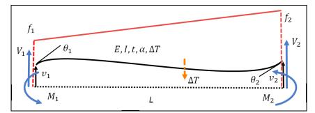
Cubic beam, linear line load, point shear forces, point bending moments, and a linear temperature decrease from top to bottom through thickness t
