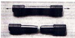
Mild ductile steel tensile test specimen
