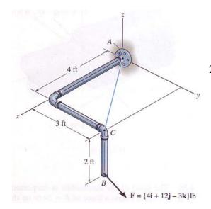
2. For the pipe assembly to the left, determine the moment of the force **F** about an axis extending between A and C. Express the result as a Cartesian vector.
