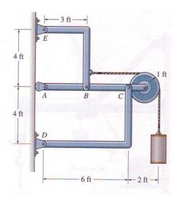
4. Determine the vertical and horizontal components of force at each pin. The suspended cylinder has a weight of 80 lb. The support at *A* is identical to a roller support.
