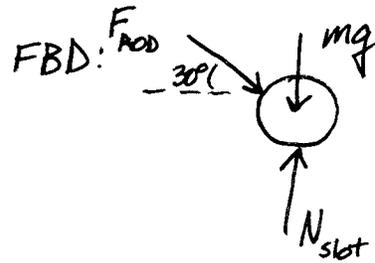
$$\Sigma F_y = N_{\text{slot}} - mg - F_{\text{rod}} \sin 30^\circ = m \ddot{y} \quad \text{b/c ball moves along slot}$$
