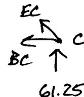
$$A) \Sigma F_y = 48.75 + \frac{3}{5}AD = 0 \rightarrow AD = -81.25 \text{ kN (c)}$$
