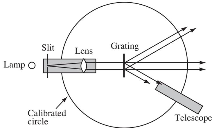
Fig. 1 Schematic diagram showing principal components of a grating spectrometer.
