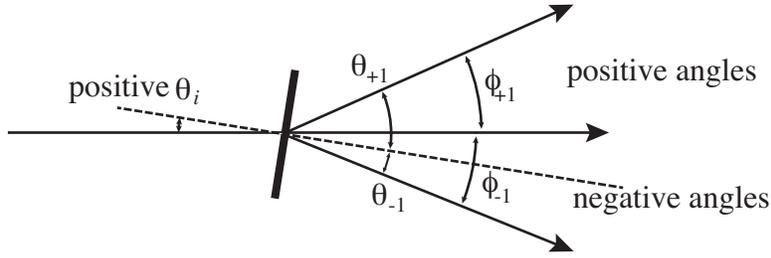
Fig. 2. Angles and sign convention for diffraction at non-normal incidence.
