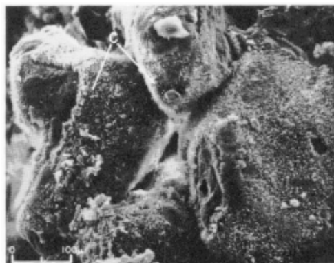
TUSCALOOSA SAND CONTAINING "PORE-LINING" CHLORITE (C) \phi = 25.7\% k_a = 41 md.
