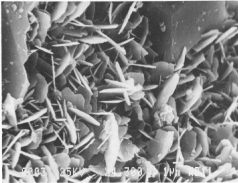
Fig. 2.13 SEM picture of grain-coating authigenic chlorite (Bjorlykke 1989)
