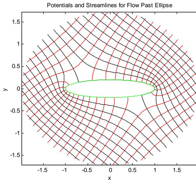
Flow past an ellipse of an inviscid fluid that is in steady translation at infinity.
