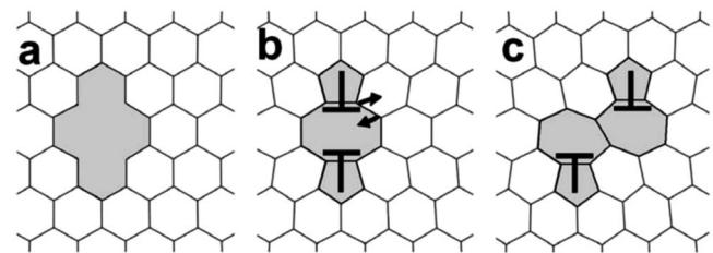
FIG. 2. Removal of two atoms creates a divacancy (a), (b), and can also be viewed as a removal of a small segment of a full crystal plane, leaving the two extra planes, that is two edge dislocations (b) able to glide away (b → c).
