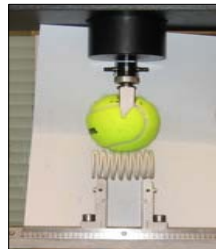
Fig. 2. Simulation of flex/ext using a tennis ball covered crosshead to distribute the force across a wide area of the sample
