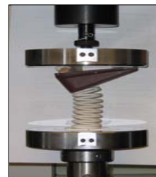
Fig. 4. Simulation of flex/ext lateral bending using an angled wedge attached to upper crosshead used to focus compressive force on one side
