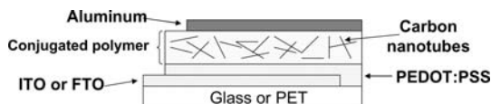
Fig. 4. Sandwich structure of bulk heterojunction organic thin-film photovoltaic cell. Glass or PET substrate is first coated with ITO or FTO, which is transparent and conductive. PEDOT:PSS is spin coated on top of the ITO to promote hole mobility into the electrode. The bulk heterojunction nanotube composite is then layered onto the device and an aluminum electrode is thermally evaporated on top of the nanotube composite [50, 51, 53–57]
