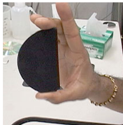
Researcher is holding paper thin battery, which can be molded into any shape
