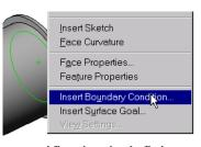
**7** Accept the default values for static pressure (101325 Pa), temperature (293.2 K) and all the other parameters.
