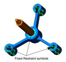
Also, a restraint icon (Restraint-1) appears in the Load/Restraint folder in the COSMOSWorks Manager tree.
