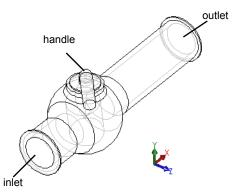
The standard engineering definition of a hydraulic resistance of an obstacle in a pipe is the difference between the total pressures (i.e. where a stream is not disturbed by the obstacle) upstream and downstream of the obstacle (the valve in our case) divided by the incoming dynamic head, from which the hydraulic resistance due to the friction over the pipe section is subtracted.
